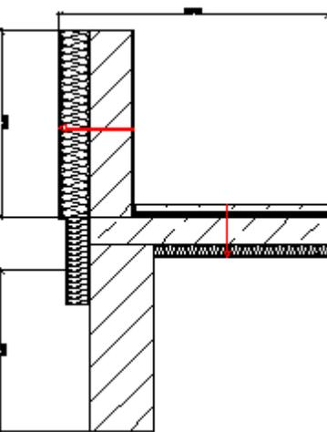
The diagram shows a cross-section of a basement wall and floor. The wall is made of masonry with diagonal hatching. Both the interior and exterior sides of the wall are insulated with a layer of insulation, indicated by red horizontal lines. The floor is a monolithic concrete slab, also indicated by diagonal hatching. A red vertical line indicates the thickness of the floor slab. The basement is unheated. |
