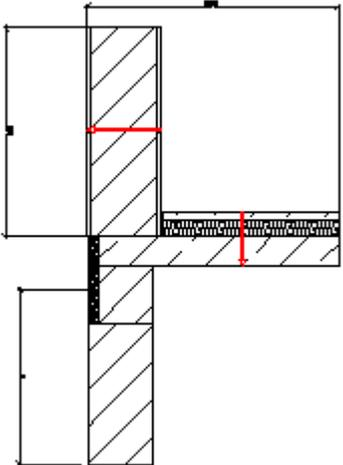
The diagram shows a cross-section of a basement wall and floor. The wall is made of masonry with diagonal hatching. The interior side of the wall is insulated with a layer of insulation, indicated by a red horizontal line. The floor is a monolithic concrete slab, also indicated by diagonal hatching. A red vertical line indicates the thickness of the floor slab. The basement is unheated.                      |
