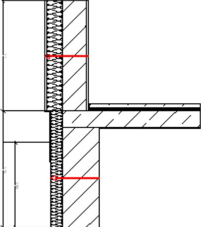
The diagram shows a cross-section of a basement wall and floor. The wall is made of masonry with diagonal hatching. The exterior side of the wall is insulated with a layer of insulation, indicated by a red horizontal line. The floor is a monolithic concrete slab, also indicated by diagonal hatching. A red vertical line indicates the thickness of the floor slab. The basement is heated.                       |
