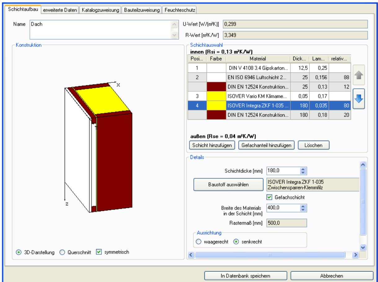
The screenshot shows the 'Schichtaufbau' software interface. The main window displays a 3D model of a roof construction with a yellow top layer and a red side layer. The interface includes several tabs: 'Schichtaufbau', 'erweiterte Daten', 'Katalogzuweisung', 'Bauteilzuweisung', and 'Feuchteschutz'. The 'Name' field is set to 'Dach'. The 'U-Wert [W/(m²K)]' is 0,299 and the 'R-Wert [m²K/W]' is 3,349. The 'Schichtauswahl' section shows a table of layers:
