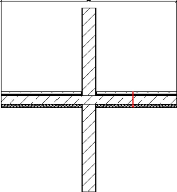
A technical cross-section drawing showing the junction of a basement floor and an interior wall. The wall is represented by a vertical hatched rectangle. The floor consists of a concrete slab (hatched with diagonal lines) and a top layer (stippled). A red vertical line is drawn on the floor slab to the right of the wall, indicating a specific detail or construction point. |
